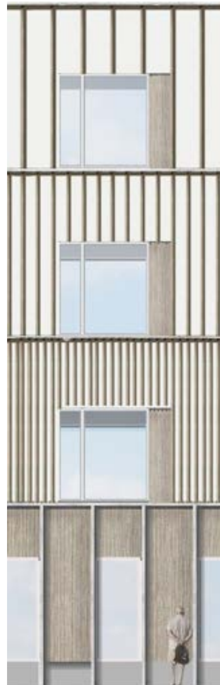
Lerketre- lameller 45 x 70 Avstand 550 mm
